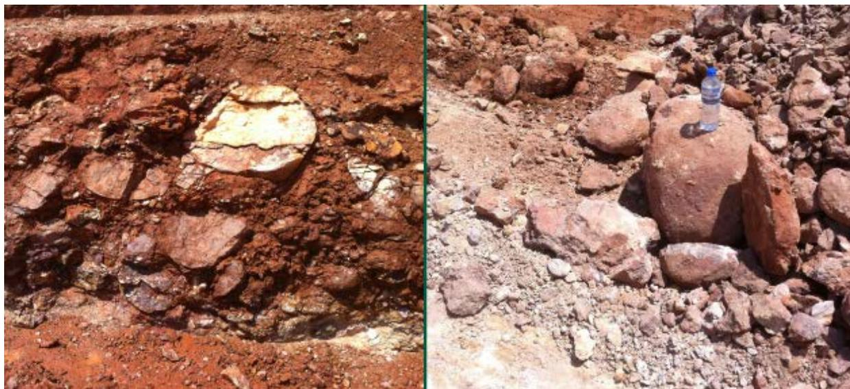
(Figure 1: Left, 1 m high gold-bearing conglomerate horizon exposed in a trench. Hard siliceous boulders and cobbles occur in a dark brown sandy matrix. Gold occurs in matrix material. Right, loosened conglomerate material collected during trench sampling. Water bottle is approximately 20 cm tall. Note that most of the siliceous boulders are free of matrix material. Screening these out may potentially help upgrade matrix material and help reduce costs of grinding in a mill.)
